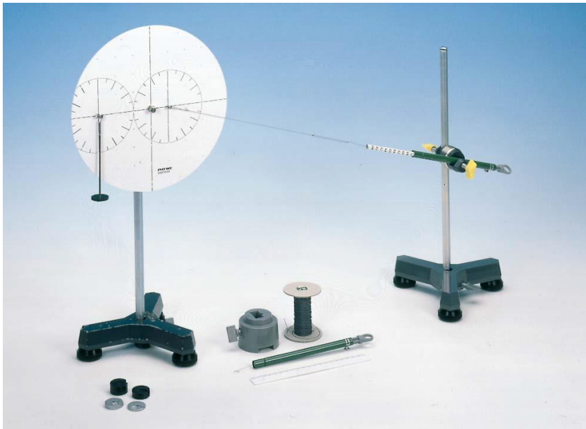
Figure 1 Experimental set-up for investigating moments in equilibrium
